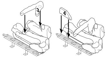
Figure 56 - Installing Log No. 3 Figure 57 - Installing Log No. 4
